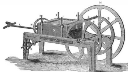
This is a superior constructed Tobacco Cut- , and they can be mo question of its qualities. ting Machine, the invention of A. P. Finch, Red Falls, Greene Co. N. Y., and is now for sale at Suydam, Reed & Co.'s, No. 108 West street, this city. Its workmanship is of a very superior kind, strong, correct and simple, be de
