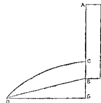
Let AB denote the height or sides of the vessel. C the hole from which the water spouts in the parabolic curve DB. Draw the line Dd and join B d so that the angles B d D shall be a right angle. Then BD is a maximum, and since the angle d B D is constant B d is a maximum, also d D. But when D d is a maximum Dd. tan.  $BDd = dB$  or  $2 AC$ . tan.  $BDd = 2 AC = AB$  or  $2 AC$  (tan.  $BDd - 1) = AB$  or  $2 AC (1 - \tan. BDd) = AB :: AC = \frac{AB}{2(1 - \tan. BDd)}$
