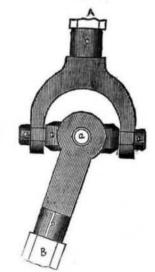
This Joint was invented by Dr. Hook, and exhibits a decided improvement over the old Universal Joint for coupling shafts that are inclined to each other This will form a useful accompaniment to the above engraving as exhibiting on an enlarged scale, the manner in which the piston rod and the connecting rod b, are united together. A and B are two shafts
