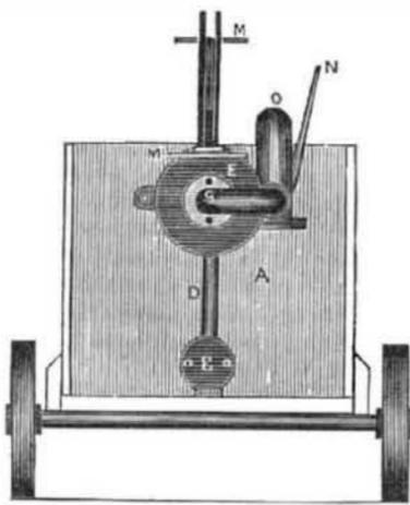
ed upon a carriage. B is the suction connecting pipe chamber. C the suction opening. D
