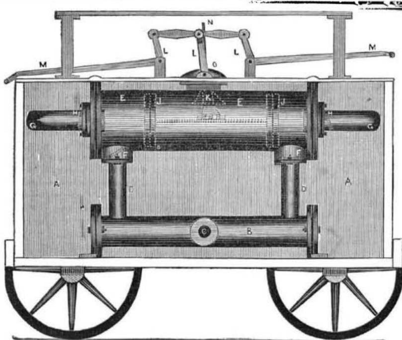
This is an invention of Messrs. Benj. Jollyn, C. Jillson and Moses Clement, of Worcester, Mass., designed for a Fire Engine and as a portable force pump,—a machine no farmer should be without.
