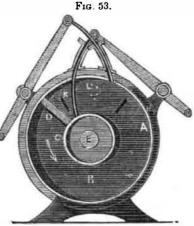
This is a vertical section of Paul Steenstrup's engine, invented in 1828, and it is a strange looking affair, yet not so curious or impracticable as to induce us to believe that only one man could conceive such an idea .-In 1847 a rotary engine nearly the same in all respects, was exhibited in New York. It is true that it was universally acknowledged to be a poor one, but still it showed that there are " many men of not many minds."
