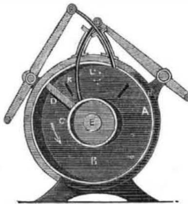
This is a vertical section of Paul Steenstrup's engine, invented in 1828, and it is a strange looking affair, yet not so curious or impracticable as to induce us to believe that only one man could conceive such an idea.—In 1847 a rotary engine nearly the same in all respects, was exhibited in New York. It is true that it was universally acknowledged to be a poor one, but still it showed that there are "many men of not many minds."
