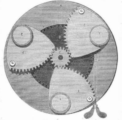
OPERATION .- The article to be operated upon being placed at or near the centre of the Chuck or axis of the pinion C, and power being applied to the screw D, turning it to the right, it will be seen that the spur wheel B, and the pinion will move towards the right from above and the pins or jaws G, being affixed to the sectors E, by a curvilinear motion approach the centre till they come in contact
