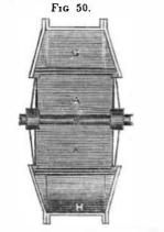
Fig. 50 is a vertical section of fig. 49 through the axis; A A, the steam wheel, B the axis, G H two valves, by which is seen their tapering figure, and the conical form of the casting which encloses them; the lower valve is shewn as closing the steam-way, and the upper one as leaving it open. It will now be perceived that the valves from this peculiar shade do not, when moving backwards or forwards, even touch the side of the casting, consequently all
