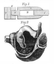
glass tube filled with percussion powder. When the point of the bullet strikes an object, the plug ignites the percussion powder in the interior, B, and the shell explodes.
