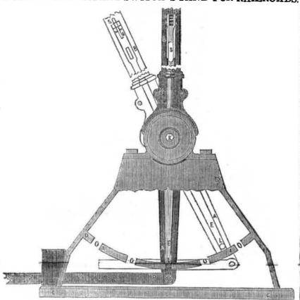
This is a Switch Stand invented by F. G. Woodward, and they are now manufactured by Mr. B. H. Goodale of Worcester, Mass. They have been highly approved by eminent engineers. This is a side view and semi-section, and shows that it is of the vertical lever kind.
