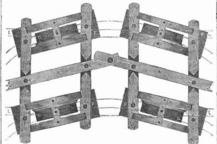
This engraving represents a very simple ar- | join two elliptical springs H, provided for each | rangement for turning short curves, invented by Mr. John H. Quail, of Philadelphia, and patented a few years ago. The curved lines is the track, and the truck is now moving over the said curve. The dotted lines L L, is the bottom frame of the car, which is attached to the truck by vertical pivots K K K, on a line of intersection with the axles. The said pivots pass through cross pieces, which
