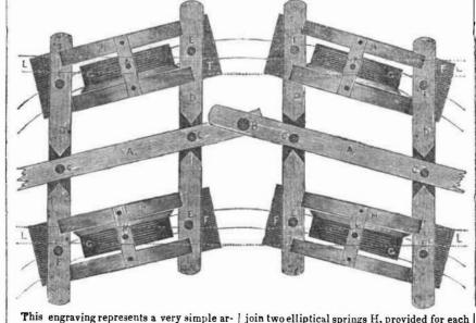
rangement for turning short curves, invented by Mr. John H. Quail, of Philadelphia, and patented a few years ago. The curved lines is the track, and the truck is now moving over the said curve. The dotted lines L L, is the bottom frame of the car, which is attached to the truck by vertical pivots K K K K, on a line of intersection with the axles. The said pivots pass through cross pieces, which
