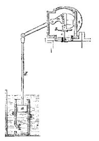
thus offered to the descent of the plunger prevents the valve dropping violently into its seat, as the water forms a graduating cushion to the descent of the plunger. At the same time, the plunger, by moving in water, enables the value to be operated almost like
