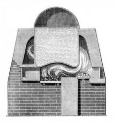
Mr. Watt observes:—"In some cases I place the fresh fuel on a grate, as at a, and beyond that grate, at or near the place where the flame passes into the flues or chimneys, I place another smaller grate, b, on which I maintain a fire of charcoal, coke or coals, which have been previously burned, until they have ceased to smoke, which by giving intense heat, and admitting some fresh air, consumes the smoke of the last fire."
