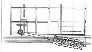
shaft is lowered so that an angle of 45° is formed, this being almost entirely destroyed the city of St. John, N. B. But considered as best adapted to allow the screw most advantageously to intercept the passing water.
