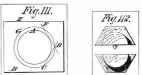
halves, letting it part across two corners, as shown in Fig. 112. When a gland of this kind is made in halves, the corners at the parting are liable, from their weakness, to chip off, and it is therefore proper to make it of hard wood.
