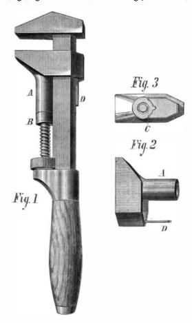
to receive the adjusting screw, which is operated in the usual way by a milled head. The rear portion of the carriage travels in a groove or channel in the bar, as indicated at C, in the horizontal section, Fig. 3.
