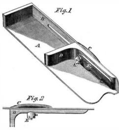
of the stationary part of the stick. By turning the lever upward, the projection is carried away from contact with the side of the slide, by which the latter is relieved from its pressure, and may then be removed to any position to adapt it to the width of the column required.
