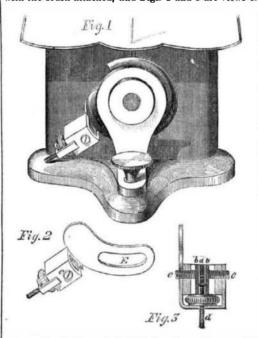
the brush and its case detached from the machine. The fine, flat hair-brush, a, is placed between two iron plates, b b, the pressure of these plates against the hair varying the rigidity of the brush, and being regulated by the screws, c c, by which also the lateral position of the brush may be adjusted. The pressure of the brush against the looper is regulated by the screw, d, and the slot, E, permits the position of the brush case to be adjusted upon the machine.
