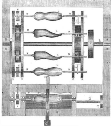
This engraving is taken from a rough model of a machine sent to us by Abner and Charles Lane, of Killingworth, Connecticut, represented to be a new invention. The motion and changing gearing is not displayed, as the model only shewed the parts.
