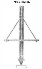
This is a representation of a Drill which is moved by pressing on the horizontal piece which is connected to the drill by bands. The drill is moved by turning the horizontal piece and when once set in motion it is alternately revolved by the action of the hand. It is just a modification of the bow drill.
