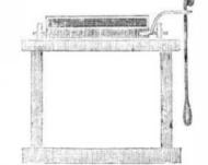
This cut represents an arrangement for giving motion to a seive by moving it backwards and forwards in the guides seen on each side at the same time that they are moved in a cross direction by the pendulum. By motion of the pendulum the box receives a kind of side to side shaking motion, while the spring on the pendulum attached to the box, gives it a longitudinal motion on the frame, thus securing two motions by the action of the pendulum.
