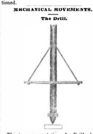
This is a representation of a Drill which is moved by pressing on the horizontal piece which is connected to the drill by bands. The drill is moved by turning the horizontal piece and when once set in motion it is alternately revolved by the action of the hand. It is just a modification of the bow drill.
