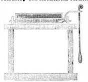
This cut represents an arrangement for giving motion to a seive by moving it backwards and forwards in the guides seen on each side at the same time that they are moved in a cross direction by the pendulum. By motion of the pendulum the box receives a kind of side to side shaking motion, while the spring on the pendulum attached to the box, gives it a longitudinal motion on the frame, thus securing two motions by the action of the pendulum.
