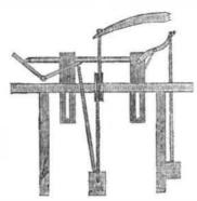
This is a machine which was proposed and used in France during the last century, invented by a gentleman named M Grandjean, for cutting screws. The piece of iron to be cut was traversed by means of the bent lever on the left which was acted on by the treadle which gives the rotary motion by the cord round the pulley. Those who would cut the head off all improvements as infringements upon old principles, have just to compare the above with modern machinery for cutting
