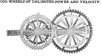
This is an arrangement of cog or toothed wheels, by which unlimited power or velocity can be obtained by means of only four wheels, and also of turning in the same or contrary directions relatively to their partners. This is an extension of Watt's highly ingenious sun and planet wheels, and is as fellows:-
