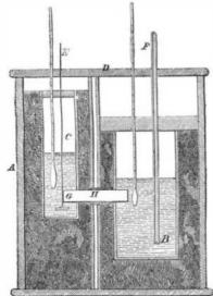
inches high. It is furnished with a cover, and painted white inside and outside. In this box are contained two square cases of vulcanized india-rubber, the sides of which are 1 an inch thick. The largest of the two cases has a length of 2 inches at each side, it is 51 inches high, and capable of containing 20 cubic inches of water. The smallest case has a length of one inch on each side, and a hight of five inches, and it is capable of containing 5 cubic inches.
