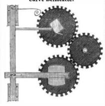
This cut exhibits a combination by which series of concentric curve lines may be described on the square surface attached to the lower wheel by means of a point proceeding from the upright part to the right, which is traversed by the upper wheel at the same time that the square surface is revolved by the
