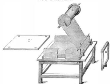
This engraving shows another mode from that described in No. 34, of obtaining a body of threads or yarns into a box in order to allow of a succession of slices or surfaces being cut off to form nap fabrics. It consists in what may be called a folding machine, whereby a warp either of one color or intermixed colors, according to the will of the party, and depending on the description of napped fabrics it is designed to produce.
