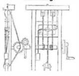
This is a front and side view of a French machine which was used some years ago for boring rifle gun barrels. Motion being given to the handle or winch, the sliding carriage which moves perpendicularly in the side guides is elevated or lowered by the inclined rope in the left hand figure, at the same time that a rotary motion is given to the perpendicular boring tool by another band passing round the horizontal warve and held tight by means of the weight.
