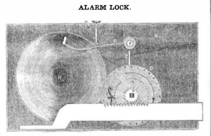
This is an invention of Mr. Wm. E. Hurlbut and Levi R. Wildman, of Danbury, Fairfield Co., Connecticut. The principle of it is the simple combination of a bell or gong with a lock, so as to strike the bell and make an alarm by turning back the bolt with a key to open the door. No other peculiarity about the lock is claimed but this.
