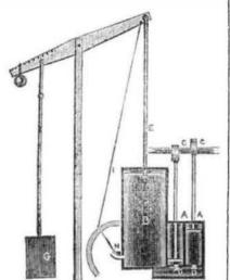
This apparatus is the invention of Mr. Jas Harvey, of Craigsville, Orange Co., N. Y .-It is the application of a double pneumatic pump to supersede the use of the governor for water wheels, especially for factories, where so much damage is often done to machinery by the breaking of some shaft, by . which the speed of looms and frames are so suddenly increased before the governor acts of any portable machine for planing metals, in arresting the speed of the main driver.
