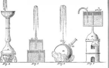
the sun to generate vapor in the upper part of the cistern, the elastic pressure of which forced the water up through the tube. The lower cistern has a pipe which leads to the upper one, in which is a valve opening upwards. A lens is made to concentrate the sun's rays upon this cistern ; the water flows into the upper one by the pressure of the vapor, and it cannot return owing to the valve in the lower pipe. Thesecontrivances never reached a higher position than curious steam toys.
