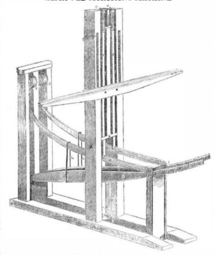
This is an important improvement on the Morticing Machine, whereby the leverage of the treadle is more perfectly adjusted to the kind of work to be morticed than by any other machine of the same kind. It is the invention of Mr. Job F. Howland, of Springfield, Mass., who has made application for a patent.
