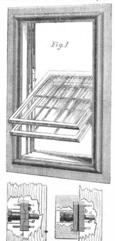
fined in the slide recess of the frame, and connected to balance cords and pulleys of the usual construction. By pushing up the window-sash, A, the strip, B, will slide up also, the same as a common sash hung on balance cords. As each window-sash is pivoted at the middle to the strip, B, it will be readily understood how is can be swung into the position shows:
