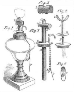
from currents of air so as to maintain a steady and uniform action, and we have been assured that a most steady and brilliant gas light is thus secured. The flame is thus raised above the top, without being depressed and drilled with a button as in the common vapor burners.
