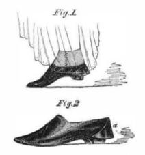
thrown up by the foot strikes against the underside of the shield; and thus the outer side, which comes in contact with the clothing, is kept perfectly dry.
