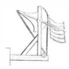
The above cut represents a method of applying the direct action of the wind and has often been proposed within the past few years somewhat modified, but the same in principle as displayed in the engraving. The plan is not very new and it altogether depends upon the vibrating action of the sector by the preponderance of the wind, or counterweight as the wind may vary.
