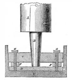
through the steel plate, C, and resting on the bottom steel plate, O, all placed in the cast iron step, E. The plates, C and D, should be bolted together with bolts, G G, and held apart by thick washers, F F. The bearing surfaces of the steel plates should be hardened and polished; and when put in motion, the step should be filled nearly full of good oil. If this step does not furnish a remedy for the evil of which he speaks, I know. of none that will. HENRY H. GUILD.
