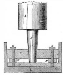
through the steel plate, C, and resting on the bottom steel plate, O. all placed in the cast iron step, E. The plates, C and D, should be bolted together with bolts, G G, and held apart by thick washers, F F. The bearing surfaces of the steel plates should be hardened and polished; and when put in motion, the step should be filled nearly full of good oil. If this step does not furnish a remedy for the evil of which he speaks, I know of none that will.
