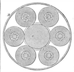
cured rigidly to the wheels, and the journal-box to the carriage. The rollers are made hollow and have the axles. dd, passing through them, which axles enter at their ends into two disks which are carried around the principal axle, A, by the rolling of the rollers, C C. In order to prevent the wear of the axles, dd, these are surrounded by sets of friction rollers as shown.
