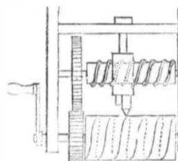
The above cut represents a method by which spirals are produced by screw movement.—The cutter is attached by a nut to a bed piece above to keep it steady as it is moved along in a slot therein. The toothed wheel on the lower shaft is driven by the handle and by said wheel meshing into the wheel on the screw axle, the cutter is moved transversely and cuts a spiral on the lower shaft as said shaft is revolved. There is a thread in the cutter box for the correct action of the screw.
