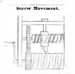
The above cut represents a method by which spirals are produced by screw movement.-The cutter is attached by a nut to abed piece above to keep it steady as it is moved along in a slot therein. The toothed wheel on the lower shaft is driven by the handle and by said wheel meshing into the wheel on the screw axle, the cutter is moved traversely and cuts a spiral on the lower shaft as said shaft is revolved. There is a thread in the cutter box for the correct action of the screw.
