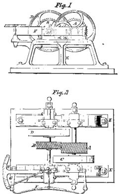
belt from the driving pulley of said working machine can be brought on the pulley, D, of the dynamometer. Another belt from the pulley, C, transmits the power to the spindle of the working machine under observation.
