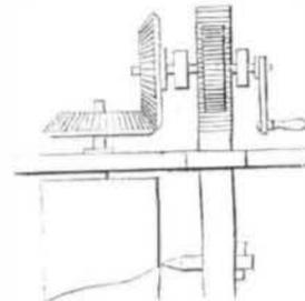
Suppose the spur wheel which gears into the perpendicular rack to be revolved by the handle on the right, the rack will be moved at the same time that the bevils will revolve the cylinder with which the horizontal bevil is connected and a regular spiral line will be described on the surface of the cylinder by the projecting point connected with the lower part of the rack.
