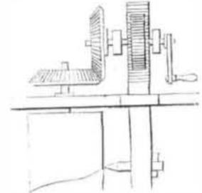
Suppose the spur wheel which gears into the perpendicular rack to be revolved by the handle on the right, the rack will be moved at the same time that the bevils will revolve the cylinder with which the horizontal bevil is connected and a regular spiral line will be described on the surface of the cylinder by the projecting point connected with the lower part of the rack.
