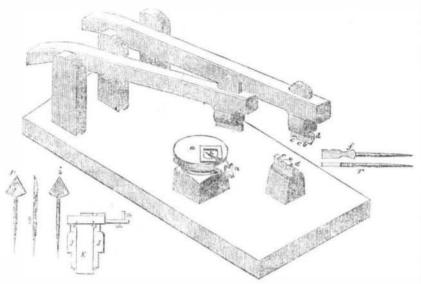
The following is a specification of Nathan Brand's patent, of Leonardsville, county of Madison, N. Y. This valuable invention is for padding hoe necks, and also can be used for other purposes. The trip hammers are here displayed of the common form of lever, but the dies and stock are adapted for the purpose set forth, and are explained by the following references to the different parts of the above engraving.
