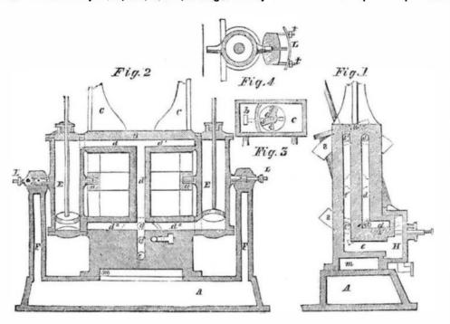
supported by hollow to communicating with the bed-plate, D, have their bearings in a long bar or yoke, F. which is bolted to the steam chest, A, so as to rise and fall with the expansions and contractions of the
