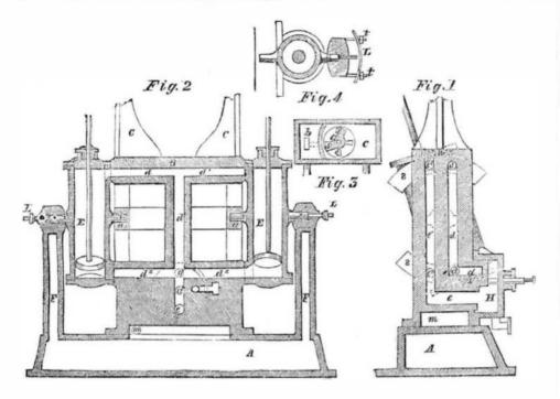
supported by hollow dependence output of the bed-plate, D, have their bearings in a long bar or yoke, F. which is bolted to the steam chest, A, so as to rise and fall with the expansions and contractions of the latter.
