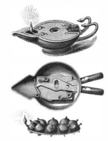
ranged that, when the handles are pressed together, the plate rotates, and one of the matches rubs against the inside of the case near the spout or opening in the cover, which rub bing or friction ignites the match and communicates fire to the ball, which thereupon burns, producing a light that lasts from five to seven minutes. This is a very curious as well as a useful little example of mechanism.
