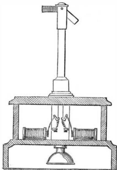
column some 18 inches high, and moves a semaphore arm at its upper extremity. Two of these arms—red and white—and two electro-magnets are employed, as represented in the engraving. On top of the case, a switch lever is arranged which serves to throw the battery current into the line wire. In front of the instrument is a tapper or ringing key for sounding the bell at the other station. The bell is shown at the lower part of the case.
