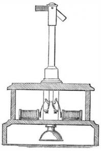
column some 18 inches high, and moves a semaphore arm at its upper extremity. Two of these arms-red and whiteand two electro-magnets are employed, as represented in the engraving. On top of the case, a switch lever is arranged which serves to throw the battery current into the line wire. In front of the instrument is a tapper or ringing key for sounding the bell at the other station. The bell is shown at the lower part of the case.
